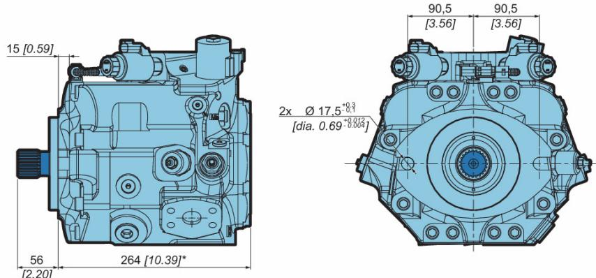
All length dimensions of pump body with different auxiliary mounting pads are shorter compare to standard 4-bolt flange of 14 mm [0.55 inch].
