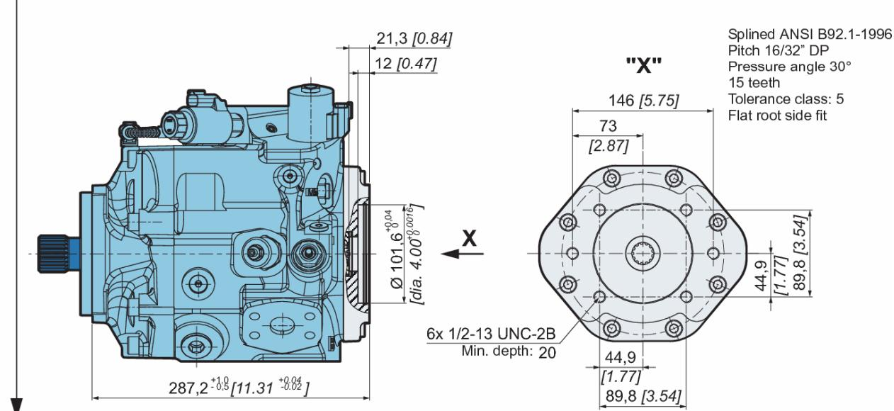
4 SAE-C; Coupling torque: 701 Nm [6204 in.lbf]; minimum active spline lenght: 14,5 mm [0.57 inch]
