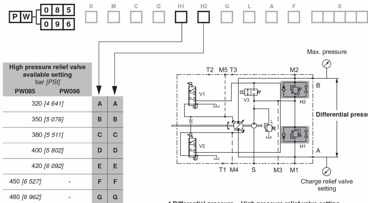
\* Differential pressure = High pressure relief valve setting
