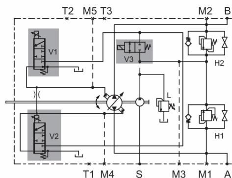
**Solenoid control with feedback sensor and cut-off valve**
