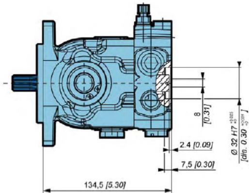
05 With charge pump: 4.9 cm<sup>3</sup>/rev [0.30 in<sup>3</sup>/rev]
