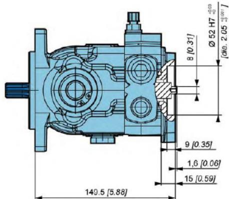
**05 With charge pump: 4.9 cm<sup>3</sup>/rev [0.30 in<sup>3</sup>/rev]**
