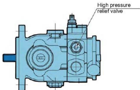
The high pressure relief valve setting is not the differential pressure between A and B ports (see page 13).
