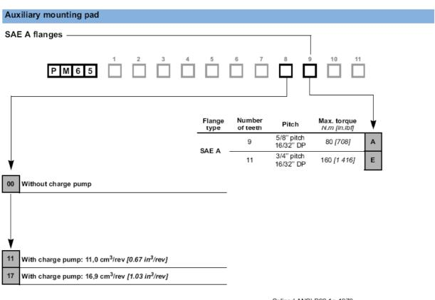
Splined ANSI B92.1a-1970 5/8" Pitch 16/32" DP Pressure angle 30° Tolerance class: 5
