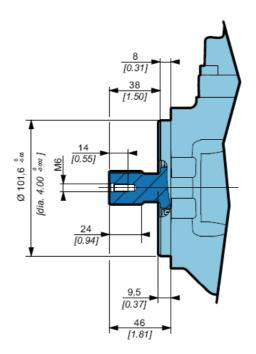
Splined ANSI B92.1a-1976 Pitch 16/32" DP Pressure angle 30° Tolerance class: 5
