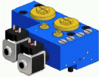
Connection block with 4LS relieves, 2 remote control connection and 2 2/2-way normally closed electrical cartridges.
